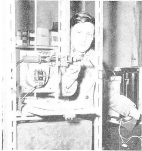
The transmitter of the Q Band signal from St. Osyth to Great Bromley. Waves are generated by the Klystron valve and emitted from the horn, centre. Wave strength is recorded
