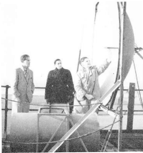
The X Band aerial on the mast. Examining the wave guide are, left to right, S. J. Masters, J. Holloway and G. C. Rider. In the rainhood, in the foreground, is the Q Band aerial. There is another at the top of the mast 360 feet up
